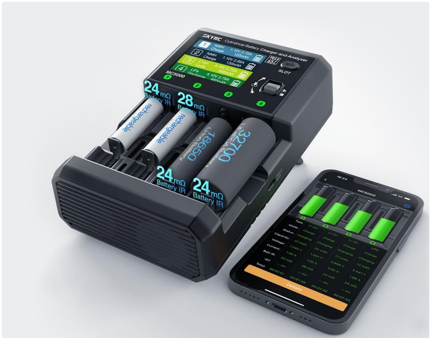
Image 3.2: The MC5000 charger shown alongside a smartphone running the SkyCharger application, demonstrating remote monitoring capabilities.
