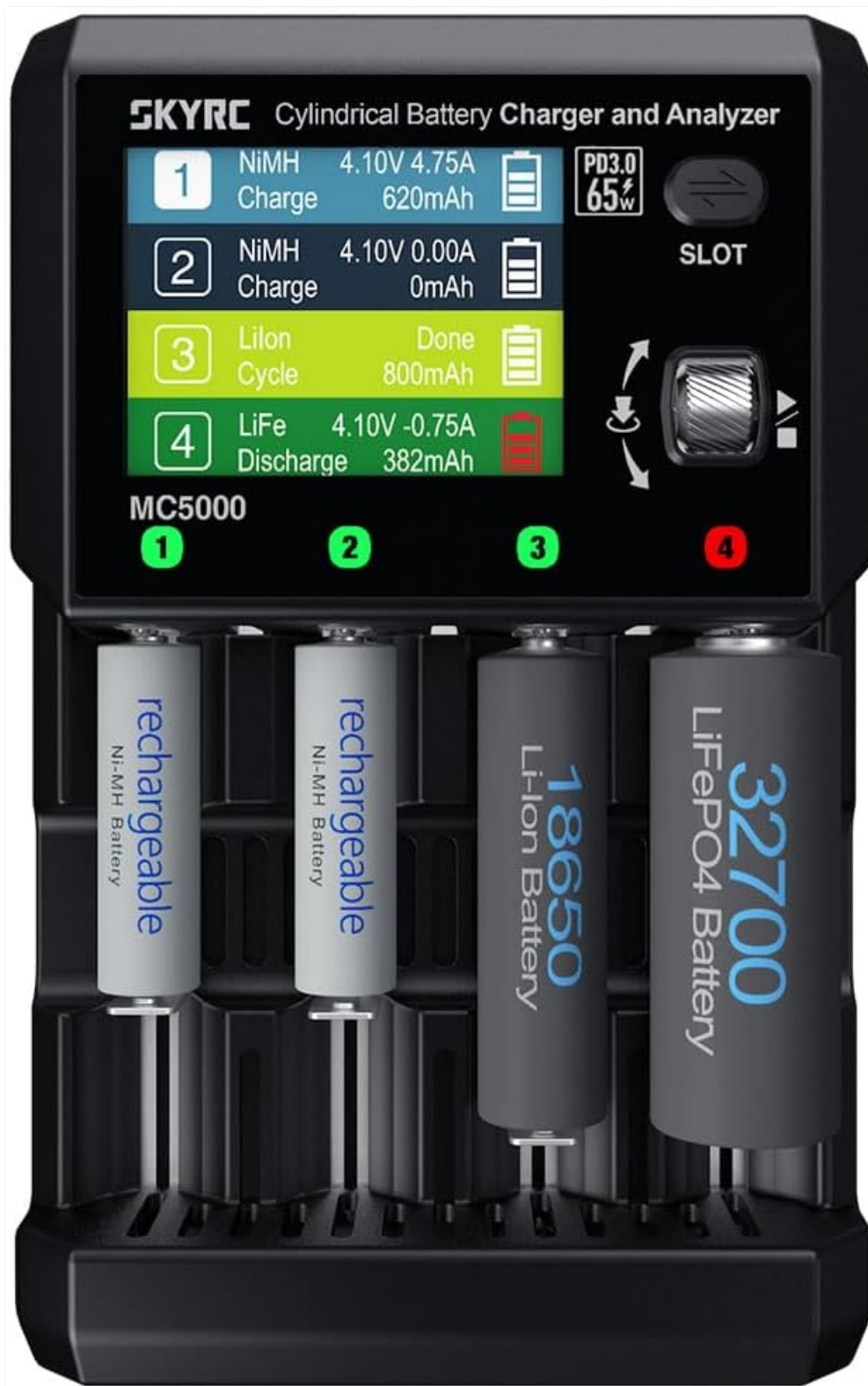
Image 1.1: The SKYRC MC5000 Cylindrical Battery Charger and Analyzer with batteries inserted, displaying operational data on its screen.
