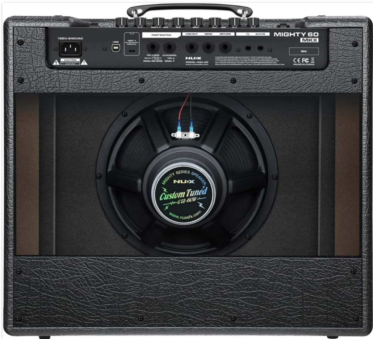
Figure 2: Rear view of the NUX Mighty 60 MKII 60-Watt Guitar Modeling Amplifier. This image highlights the various input/output jacks, power connection, USB port, footswitch input, and the custom-tuned speaker (Model: NGA-60, WV-G12-60W).
