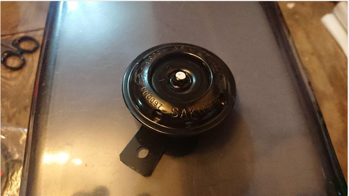
Figure 3.1: SAKURA AH-368 Horn Unit. This image shows the compact black horn with its integrated metal mounting bracket, ready for installation.
