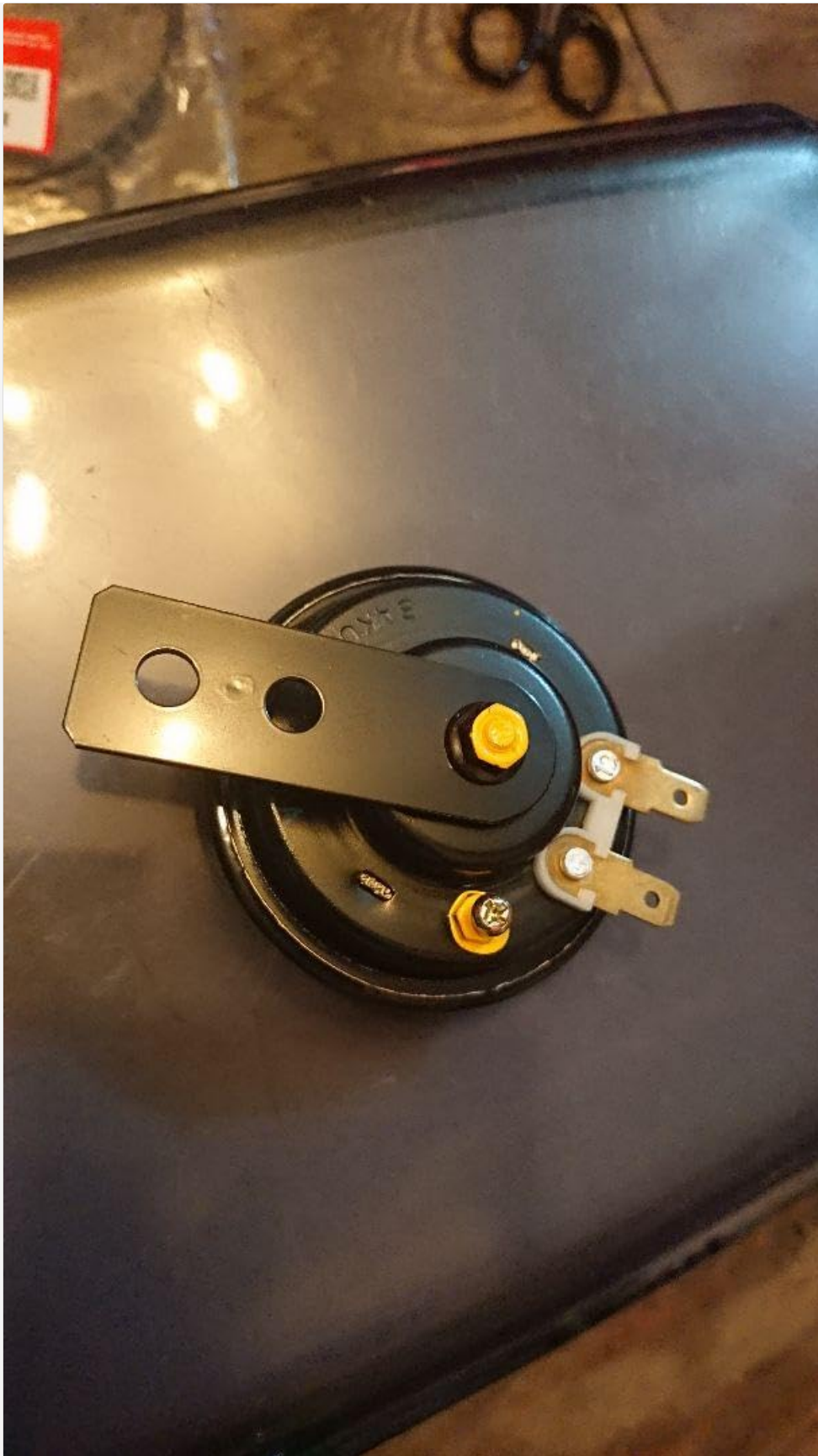
Figure 5.1: Horn Electrical Terminals. This image displays the back of the horn, highlighting the two terminals where electrical connections are made for power and ground.
