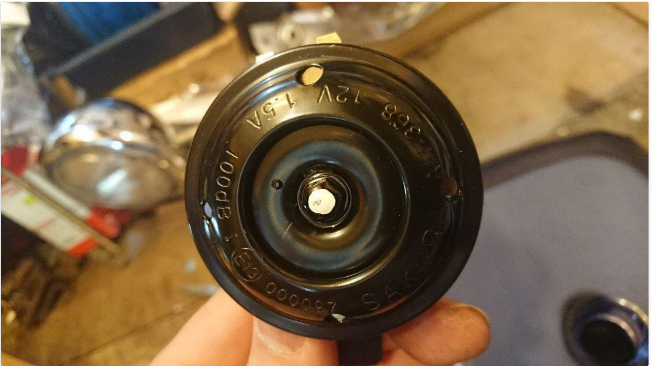
Figure 4.1: Horn Specifications Detail. This image provides a close-up of the horn's face, clearly displaying the voltage, current, and decibel ratings.
