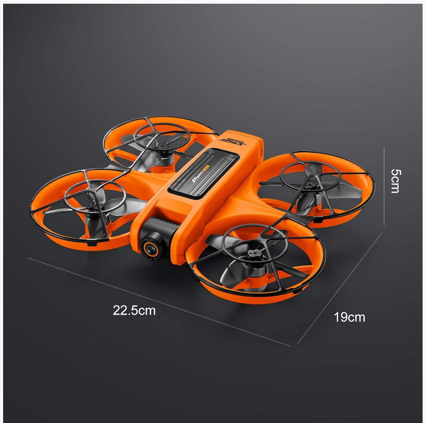
Image 3.2: The SuperRC S156 drone with its approximate dimensions: 22.5cm length, 19cm width, and 5cm height.
