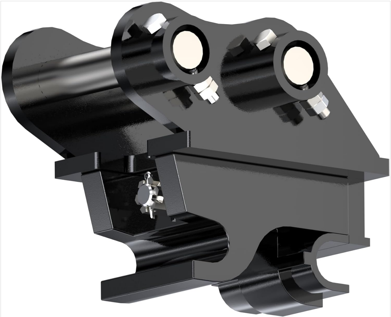
Figure 3.2.1: Quick Hitch with key dimensions. The main pin diameter is 25mm, and the internal width is 93mm. The mounting plate thickness is 10mm.
