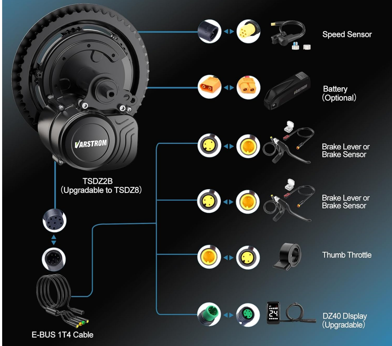
Image 4.1: Diagram illustrating the connections for the motor, speed sensor, battery, brake levers/sensors, thumb throttle, and display.
