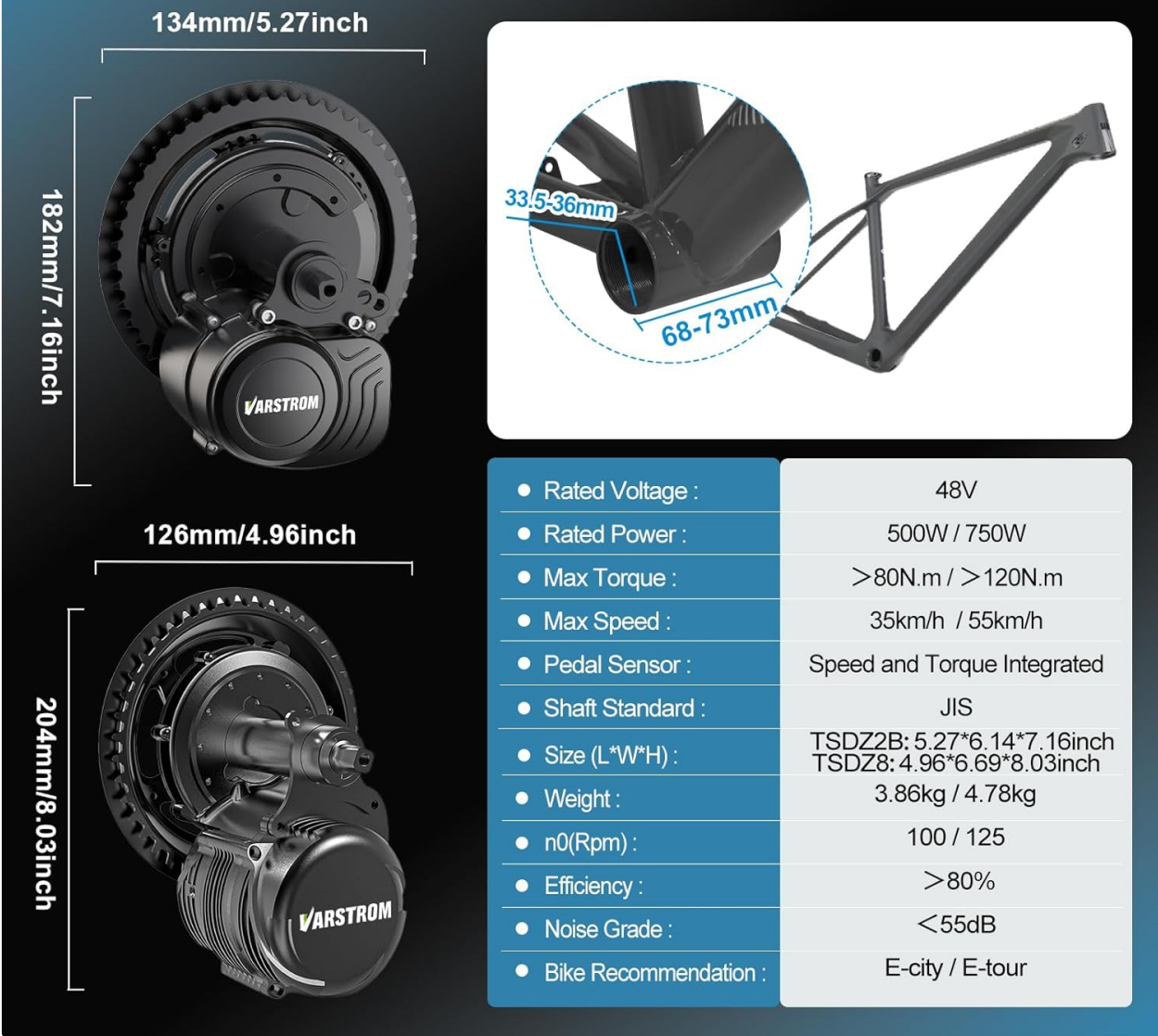
Image 3.2: Motor dimensions and detailed specifications for compatibility.
