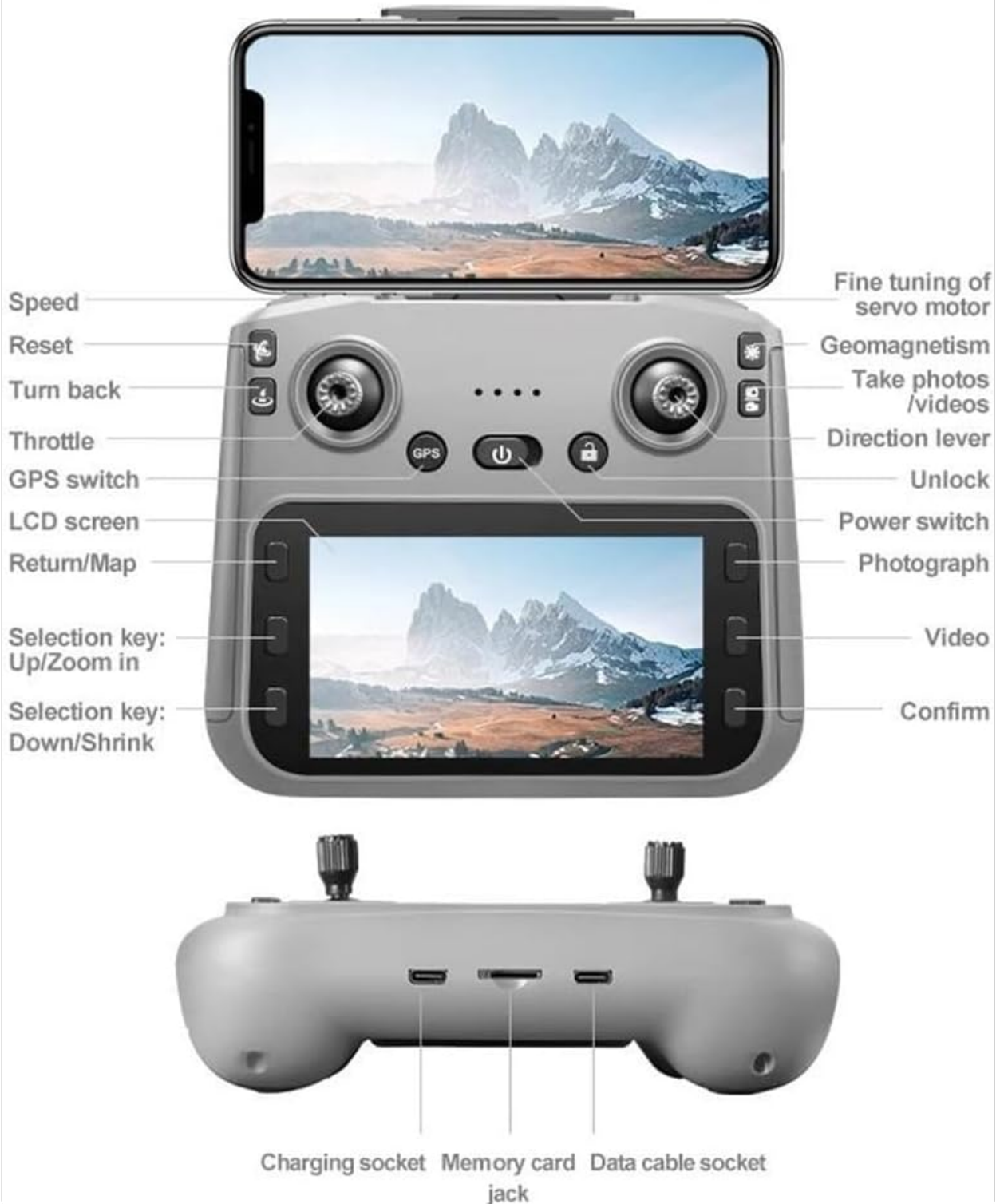
Figure 4.2: Detailed diagram of the remote control with labeled buttons and ports.
