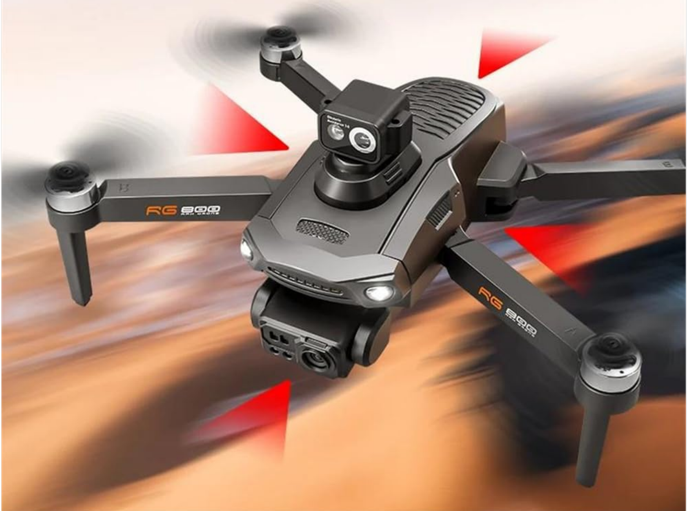
Image 3: The drone illustrating its four-sided obstacle avoidance system, which helps in detecting and guarding against collisions from various directions during flight.
