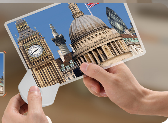
Figure 4.3: The corner rounder tool providing smooth, rounded edges to a laminated item.
