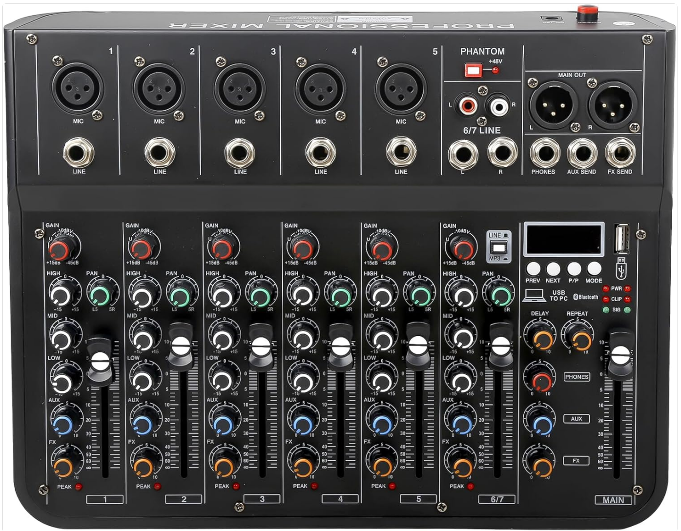
Figure 1: Top view of the jindaudio 7-Channel Audio Mixer. This image displays the microphone/line inputs, main output, headphone jack, USB port, Bluetooth indicator, and various control knobs for gain, equalization (high, mid, low), pan, effects (delay, repeat), and main volume faders.
