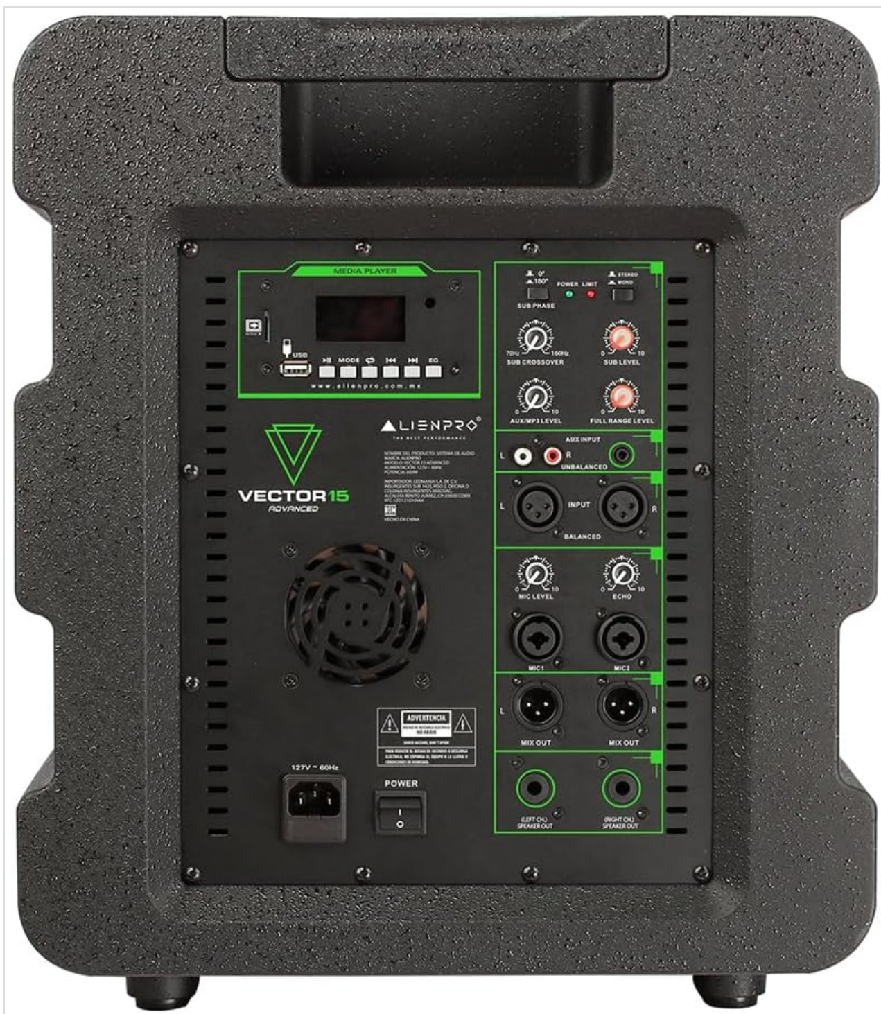
Figure 7: Subwoofer Rear Panel Controls and Connections.
