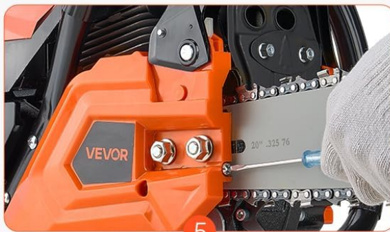
Close the side cover, adjust the chain tension, and ensure the distance between the chain bottom and guide bar is 2-4 mm
