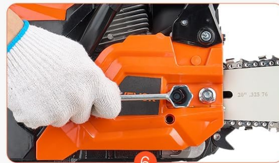
Install the chainsaw, ensuring the direction of the teeth is correct
