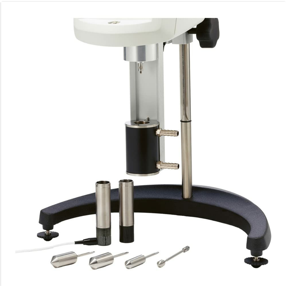
Figure 1: Components of the AMETEK Brookfield Small Sample Adapter SSA 18/13R. This image displays the main viscometer unit with its stand, a black cylindrical water jacket attached to the viscometer shaft, two silver cylindrical sample chambers, and four different conical spindles. The water jacket features two barbed fittings for connecting to an external circulating bath.
