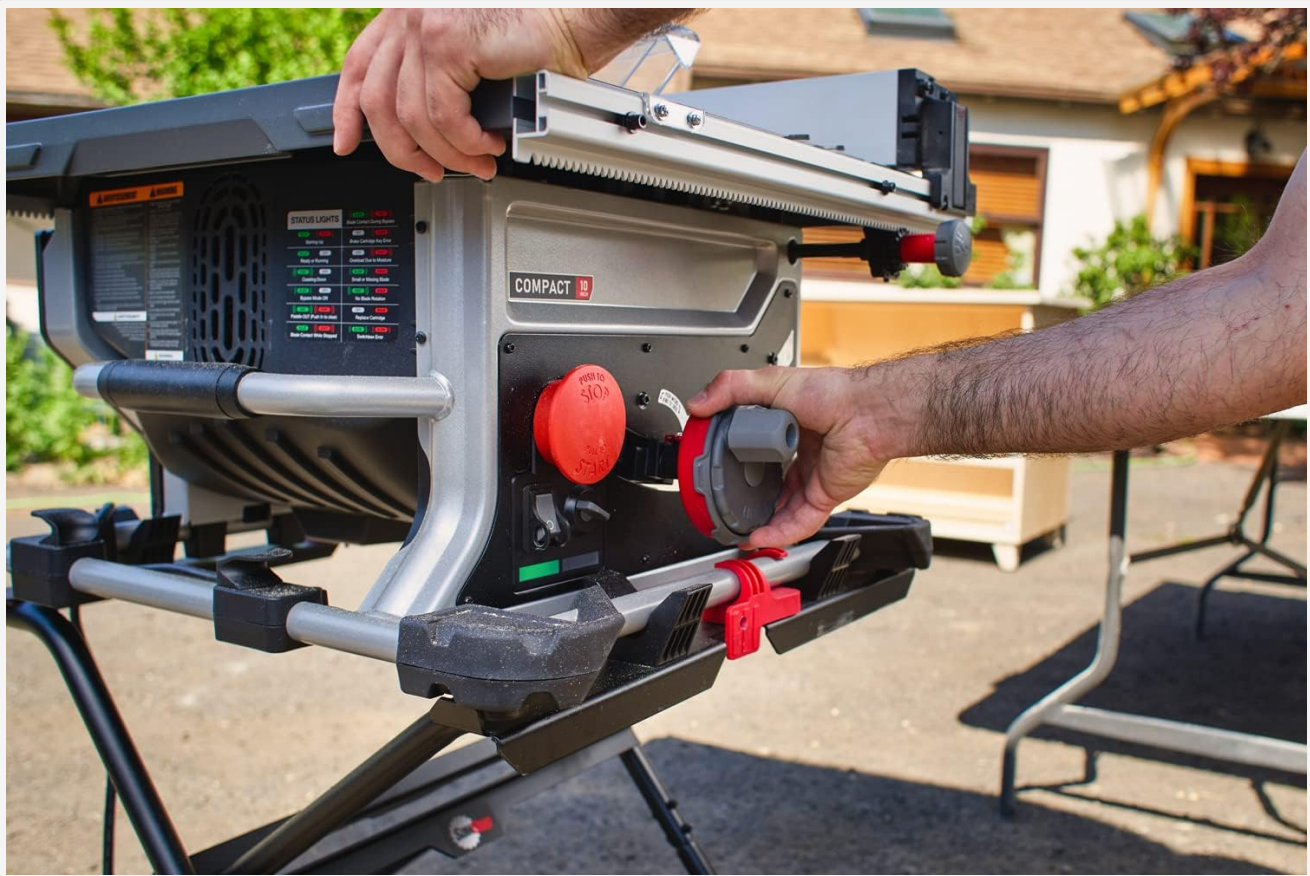
Figure 4.1: Adjusting the blade height and angle using the saw's control knobs.
