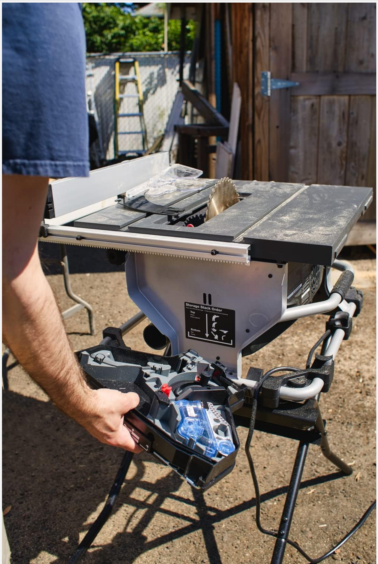
Figure 5.1: Process of removing the SawStop safety cartridge for inspection or replacement.
