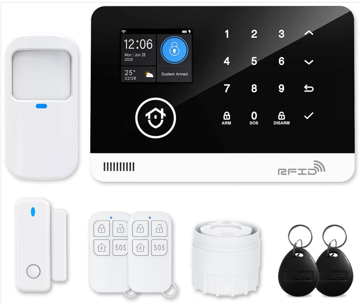
Image 2.1: The complete TUGARD Smart Home Security Alarm System 8-piece kit, including the control panel, motion sensor, door/window sensor, remote controls, RFID tags, and siren.
