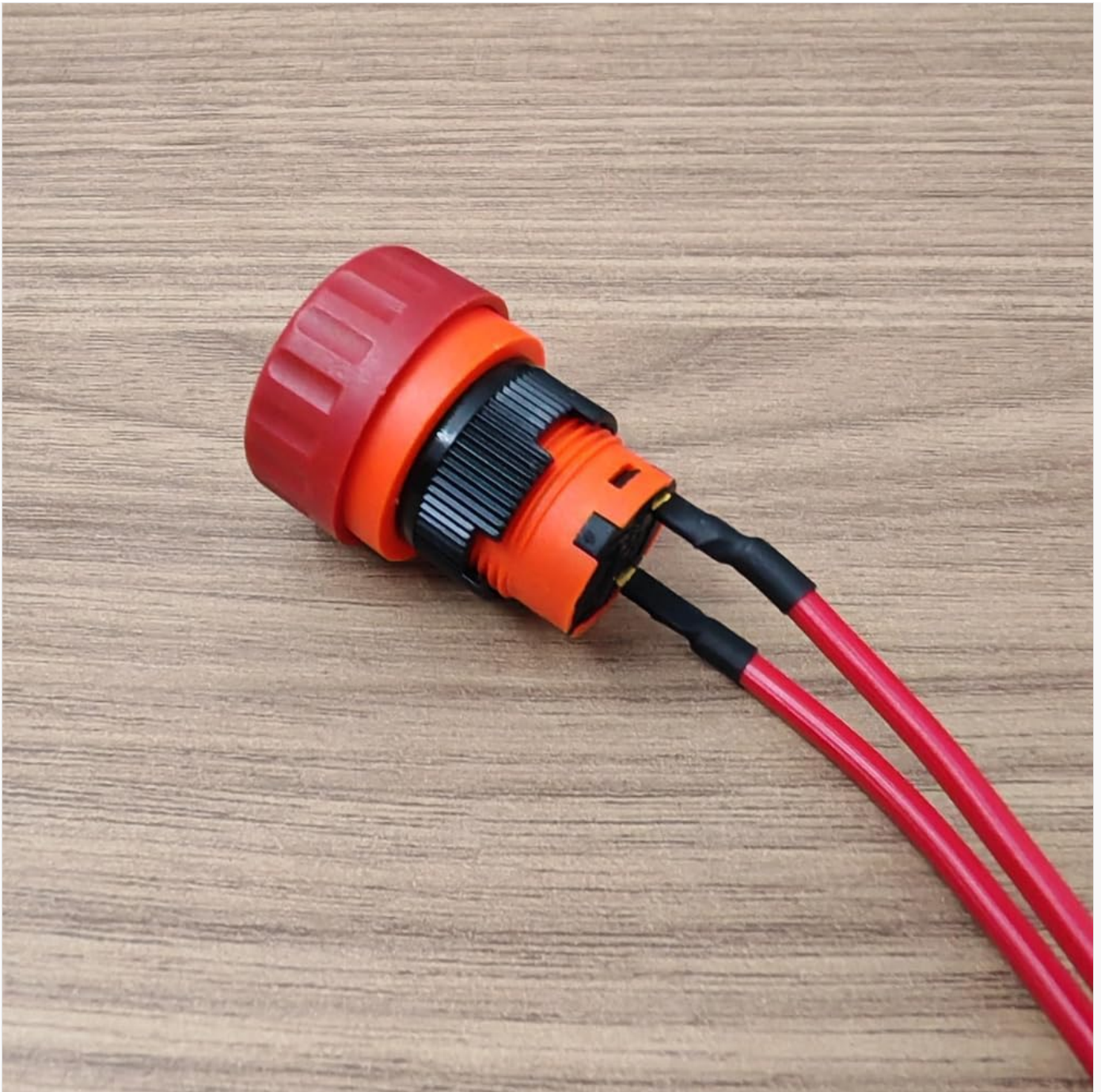
Figure 2: Rear view of the emergency stop switch, illustrating the terminal connections and the mounting nut. The two red wires are pre-attached to the SPST (Single Pole Single Throw) Normally Closed contacts.
