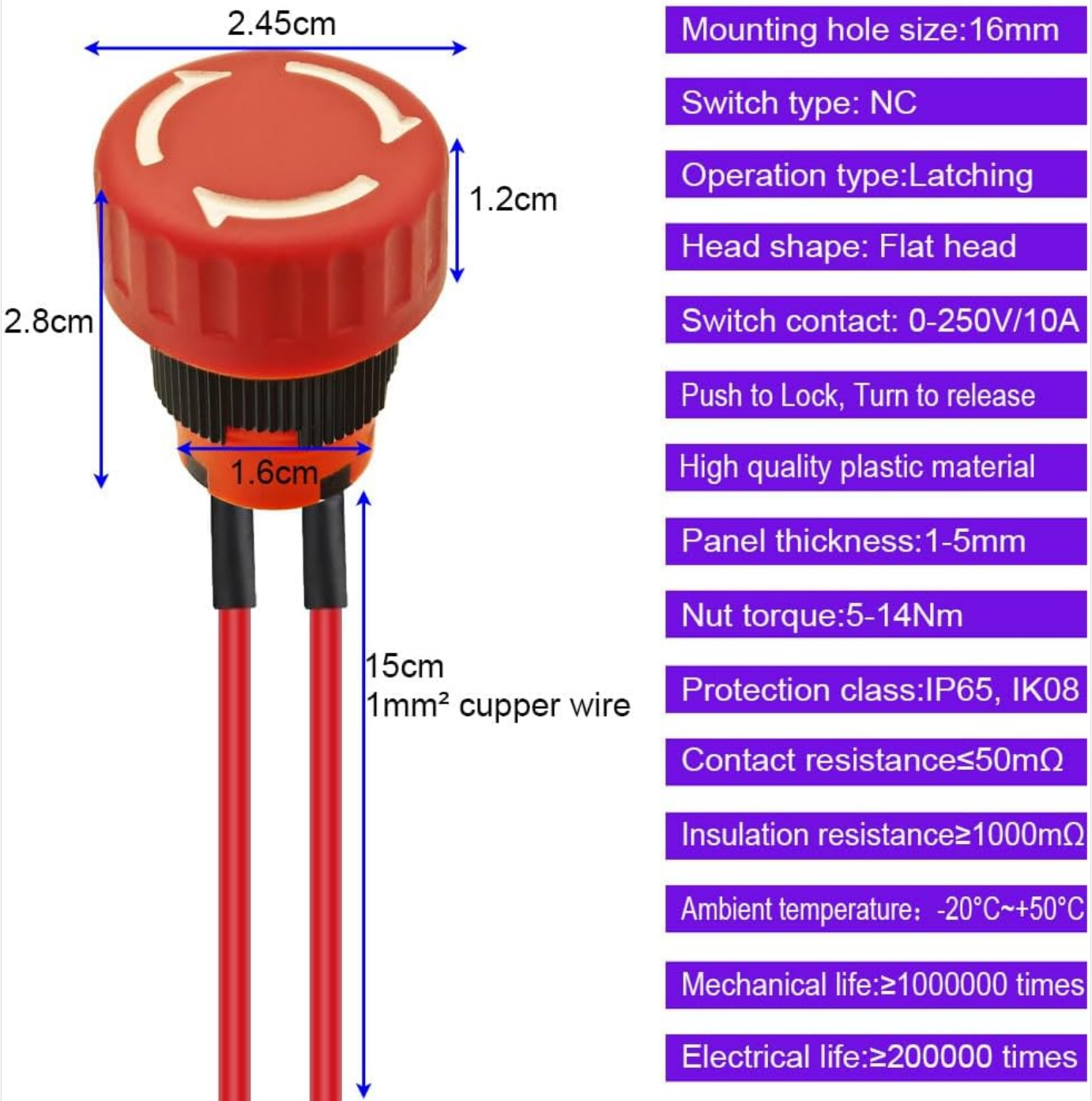
Figure 3: Detailed diagram of the emergency stop switch with key dimensions (e.g., head diameter, mounting hole size) and technical specifications.
