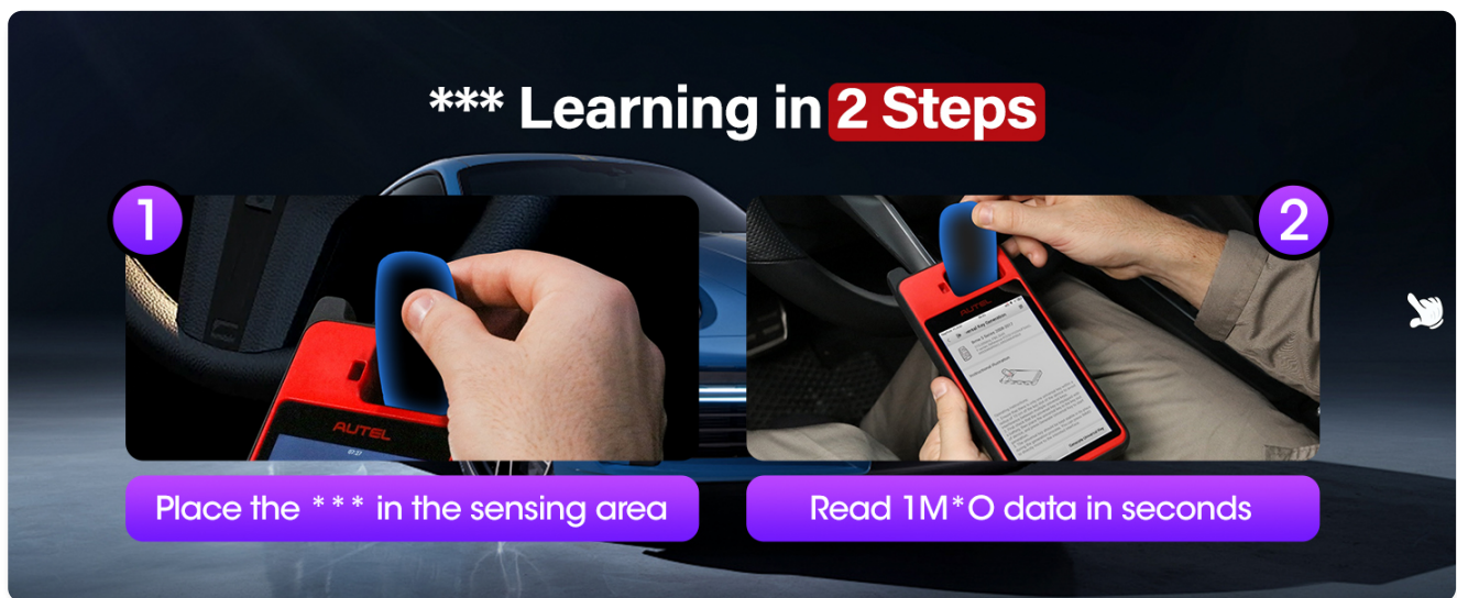
Image 4.2: Simplified two-step key learning process using the KM100X.
