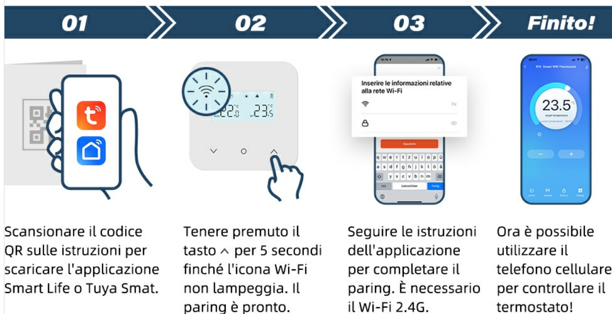
Image 3.3.1: Visual guide for connecting the thermostat to the mobile app. Step 1 shows scanning a QR code for app download. Step 2 shows activating Wi-Fi pairing mode on the thermostat. Step 3 shows entering Wi-Fi information in the app. The final step shows the app interface controlling the thermostat.
