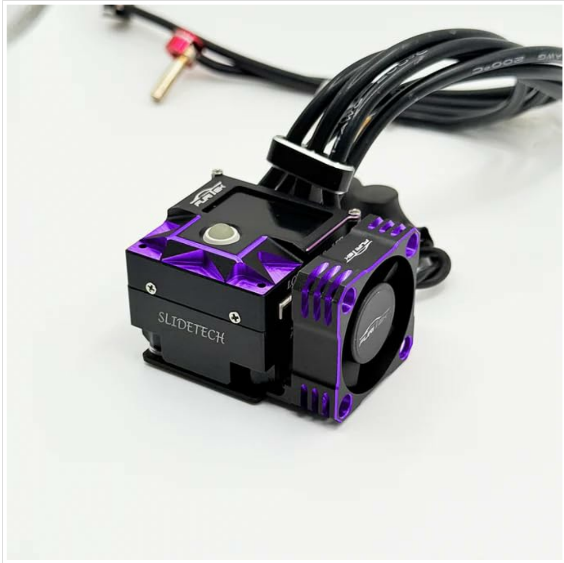
Image: The Furitek AeroSpin 30K fan kit fully installed on a SlideTech ESC, showing the side profile and connection points.
