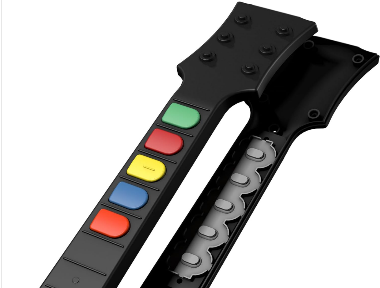
Image: An internal view of the guitar controller's neck, highlighting the classic rubber membrane fret buttons designed for an authentic feel.
