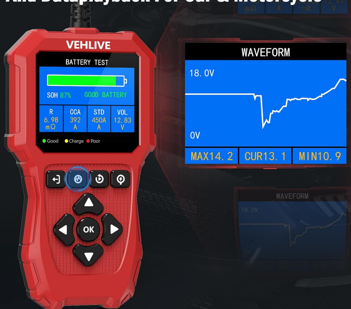
Figure 6: The BT910 screen showing detailed battery test results, including SOH, internal resistance, CCA, and voltage, alongside a real-time voltage waveform analysis.
