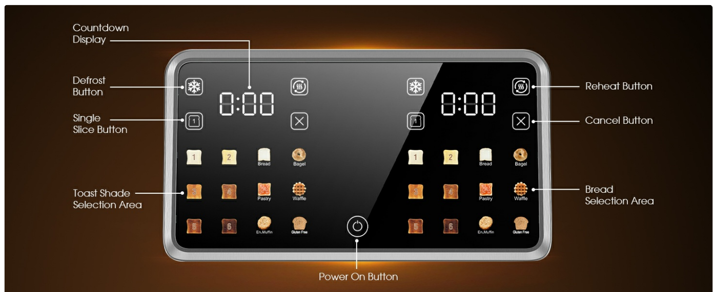
Image: Diagram illustrating the various buttons and indicators on the toaster's touch screen, including Countdown Display, Defrost Button, Single Slice Button, Toast Shade Selection Area, Power On Button, Reheat Button, Cancel Button, and Bread Selection Area.
