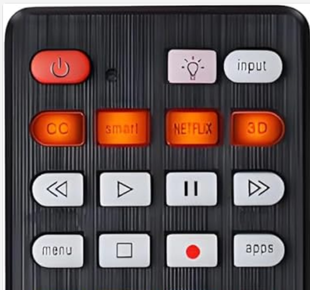
Image: Close-up of the remote control, emphasizing the fluorescent buttons that glow for better visibility in low light.
