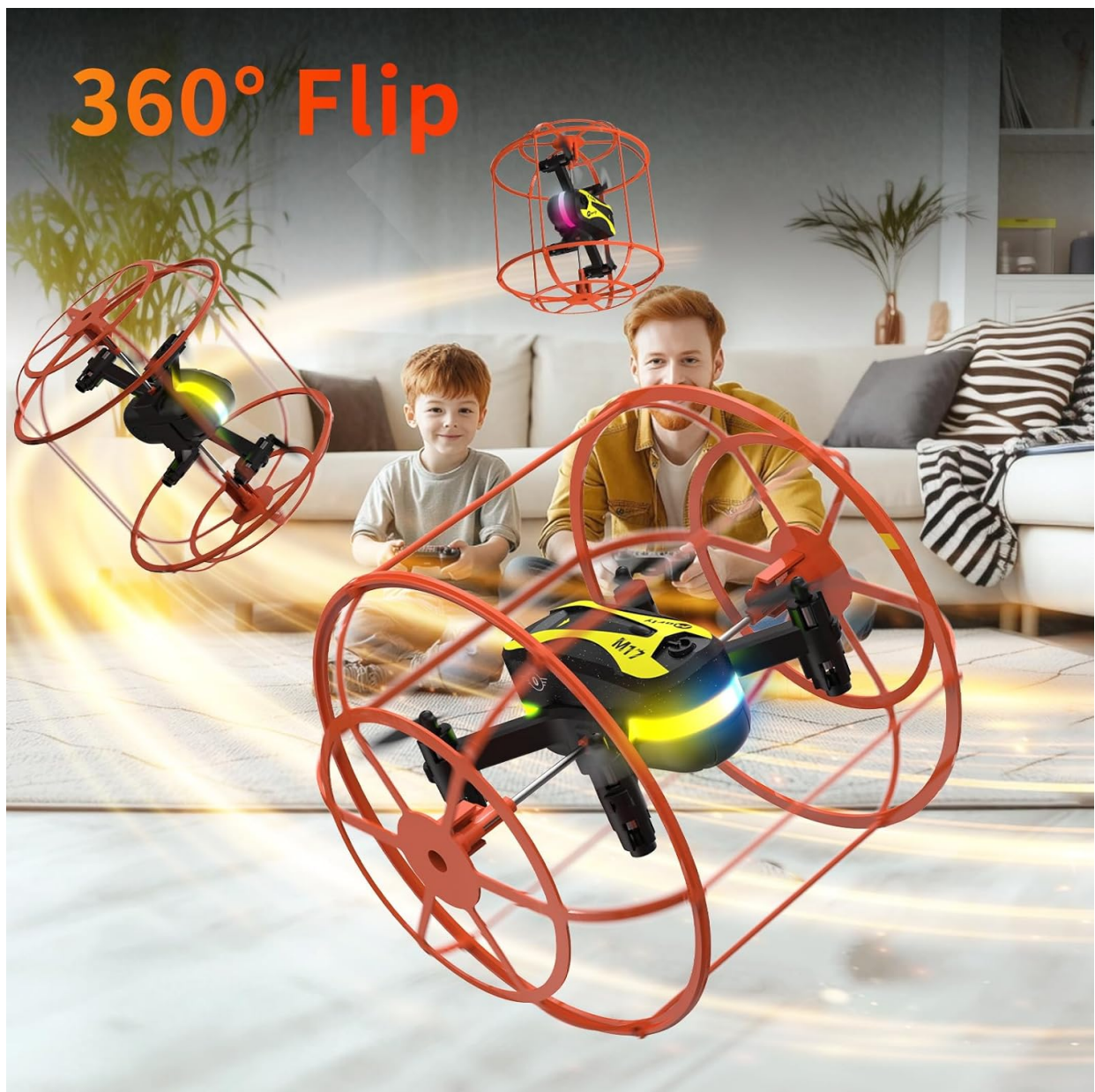
Figure 6: The M17 Mini Drone executing a dynamic 360-degree flip, a fun feature for experienced pilots. To perform a 3D flip, press the 3D flip button on the controller, then quickly move the right joystick in the desired flip direction (forward, backward, left, or right).
