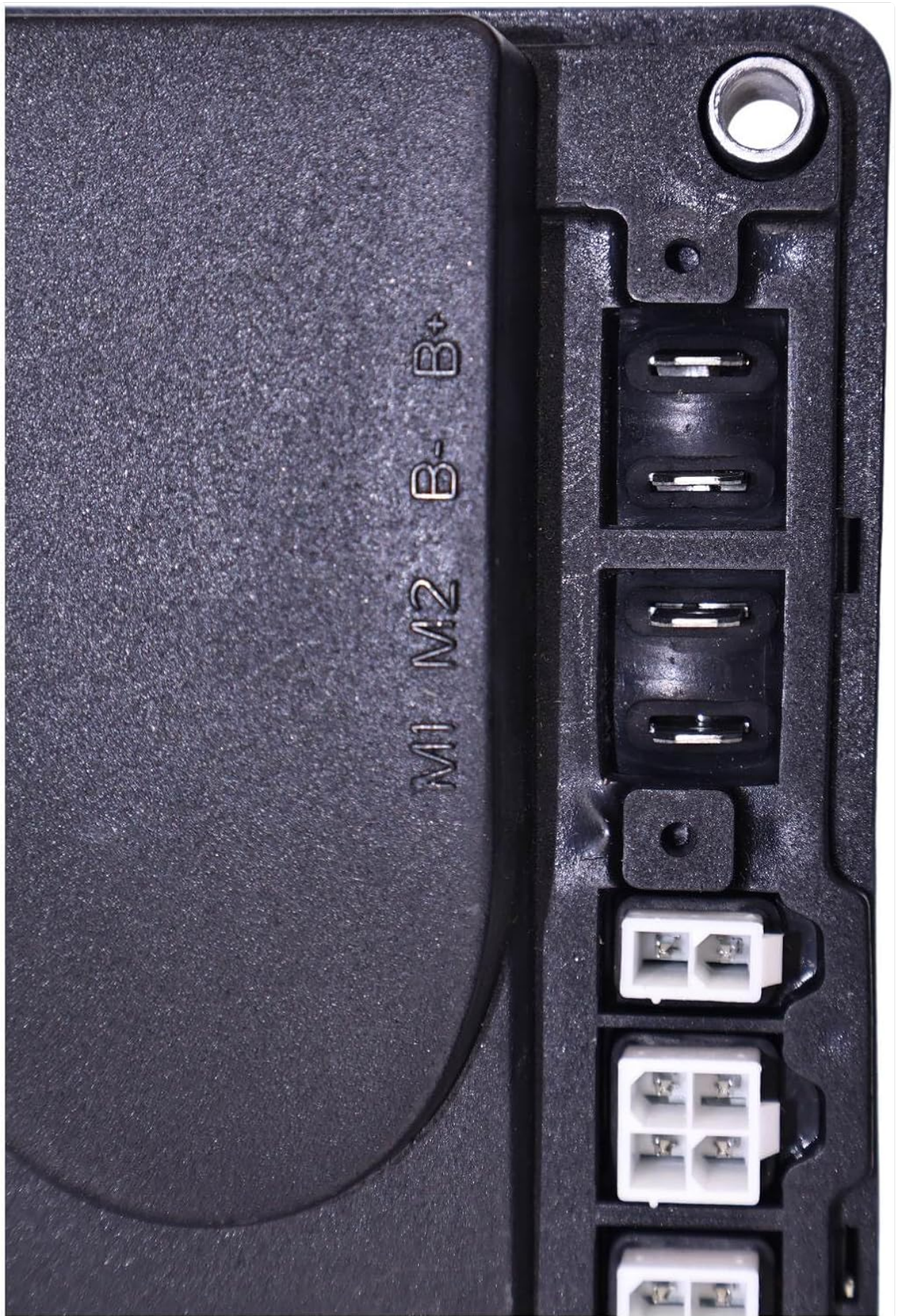
Image: Close-up of the larger metal terminals on the controller, clearly labeled M1, M2, B-, and B+. These are the main power and motor connections.
