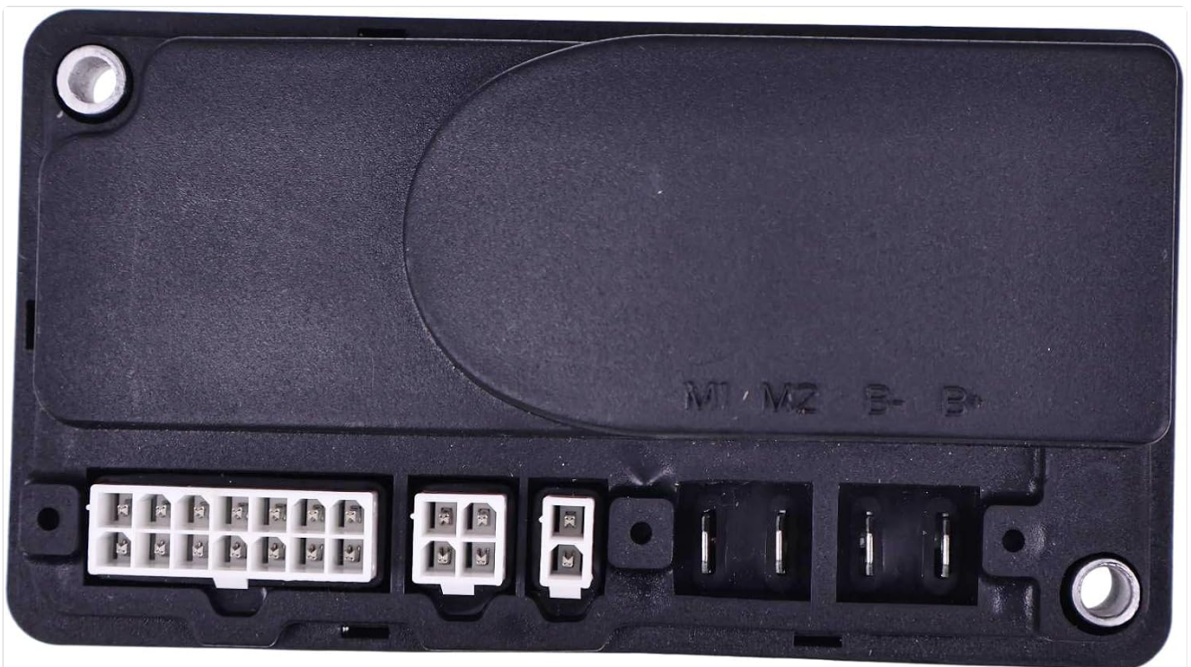
Image: Top-down view of the controller, highlighting the various white multi-pin connectors and larger metal terminals for power connections. Markings like M1, M2, B-, B+ are visible near the terminals.
