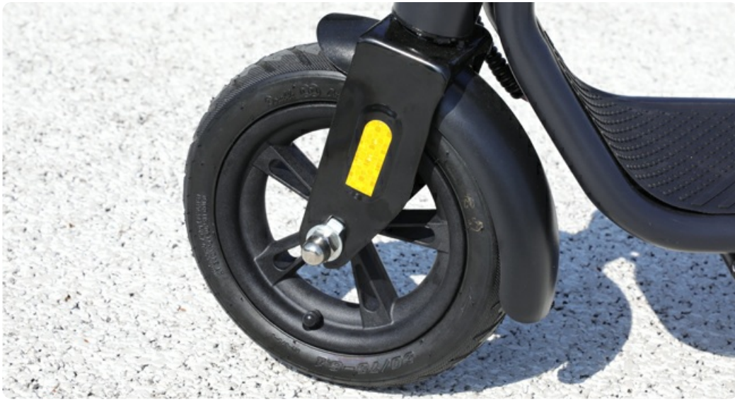
Image: A close-up of the front pneumatic wheel, highlighting its shock-absorbing capabilities for a comfortable ride.
