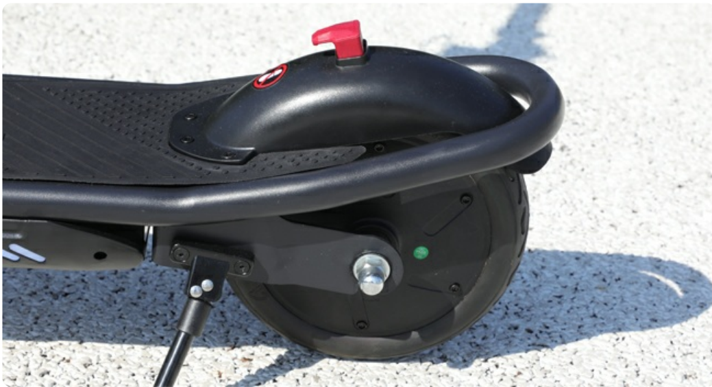
Image: A close-up of the rear solid motor wheel, emphasizing its anti-flat design and low maintenance requirement.
