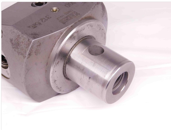
This image displays the mounting shank of the boring head, which connects to the machine spindle, and the internal threading for securing the boring bar.
