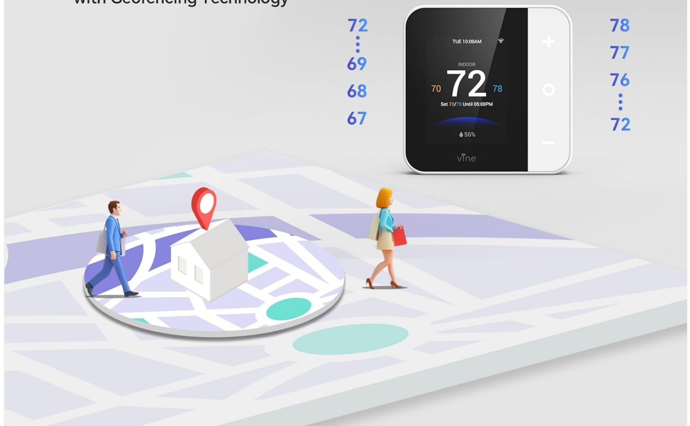
Figure 7.4: Geofencing feature automatically adjusts thermostat settings as you enter or leave a predefined area.
