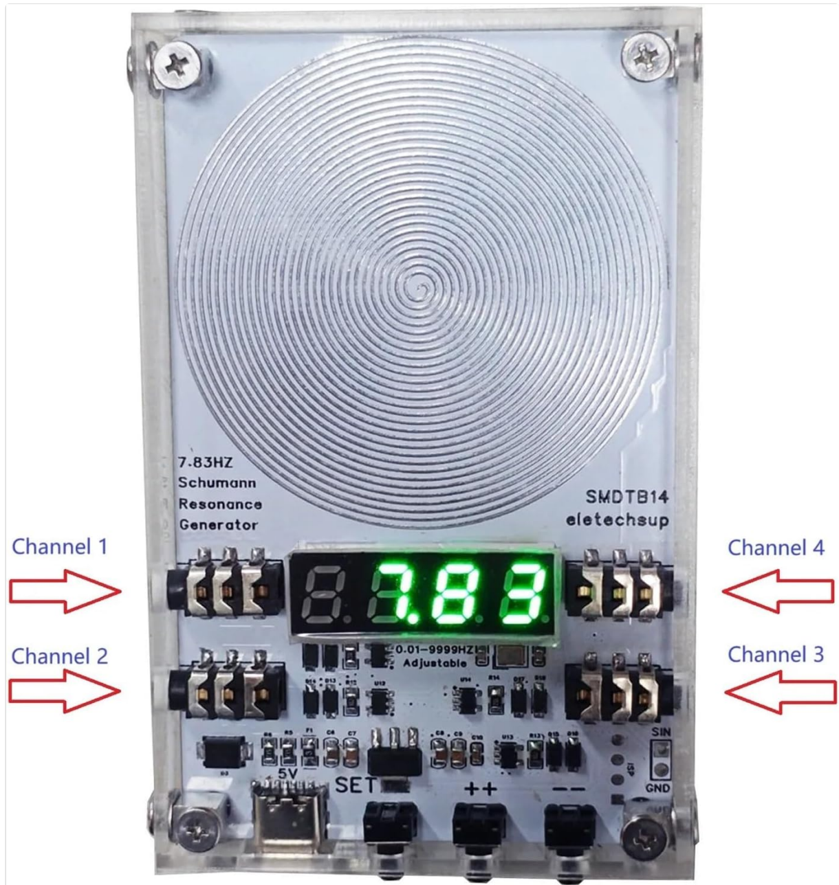
Figure 3: The SMDTB14 signal generator highlighting its four independent audio output channels (Channel 1, Channel 2, Channel 3, Channel 4) for connecting external antennas.
