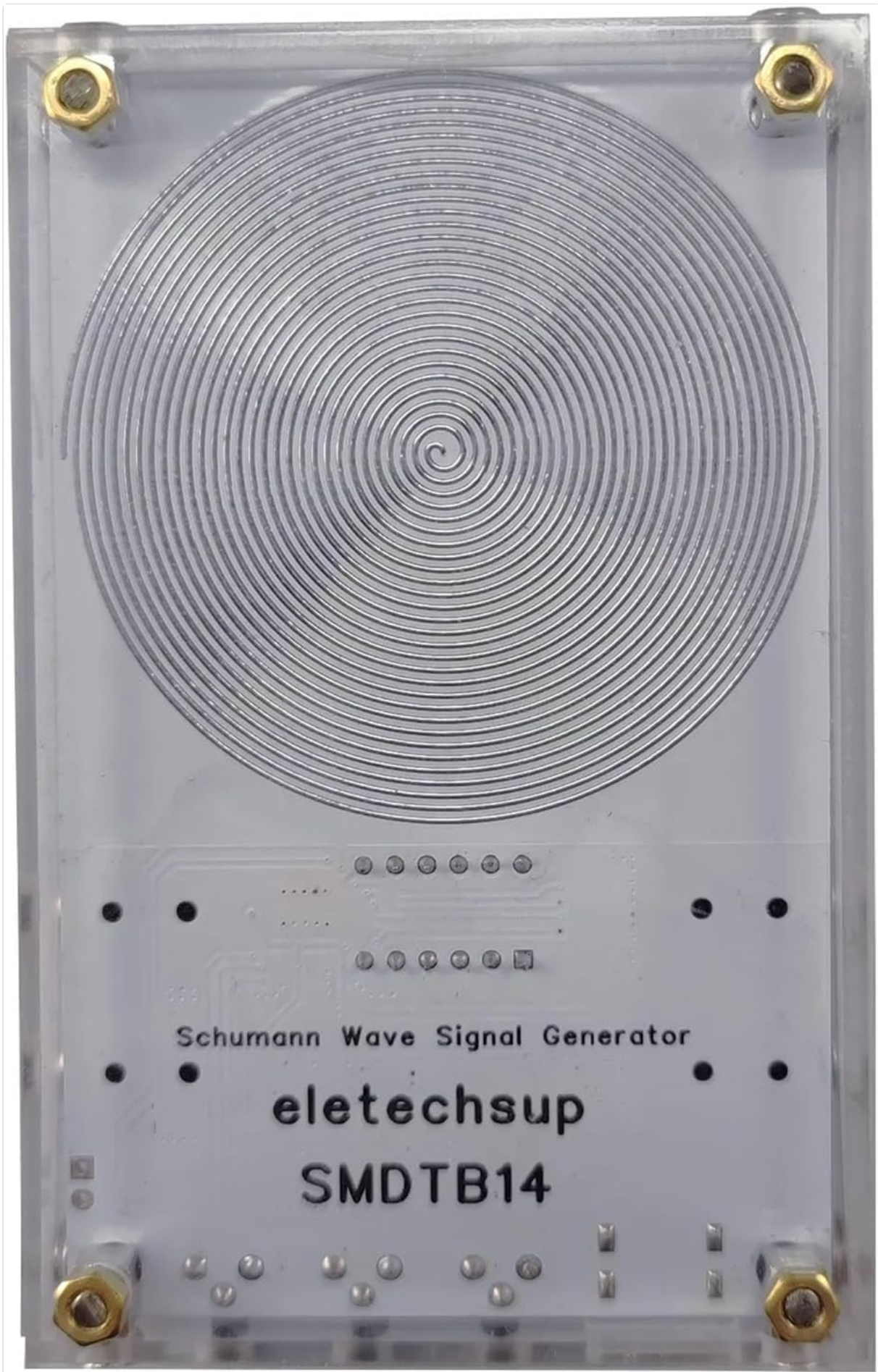
Figure 5: Top view of the SMDTB14 circuit board, showing the spiral antenna design and the 'Schumann Wave Signal Generator' and 'eletechsup SMDTB14' labels.
