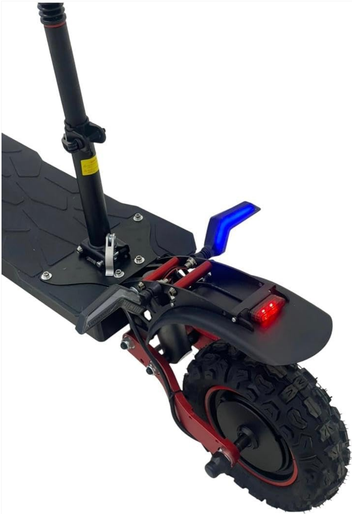
Image 5.2: Rear section of the scooter, showing the brake light, fender, and robust rear wheel.
