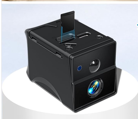
Figure 3.1: Location of the MicroSD card slot on the camera.
