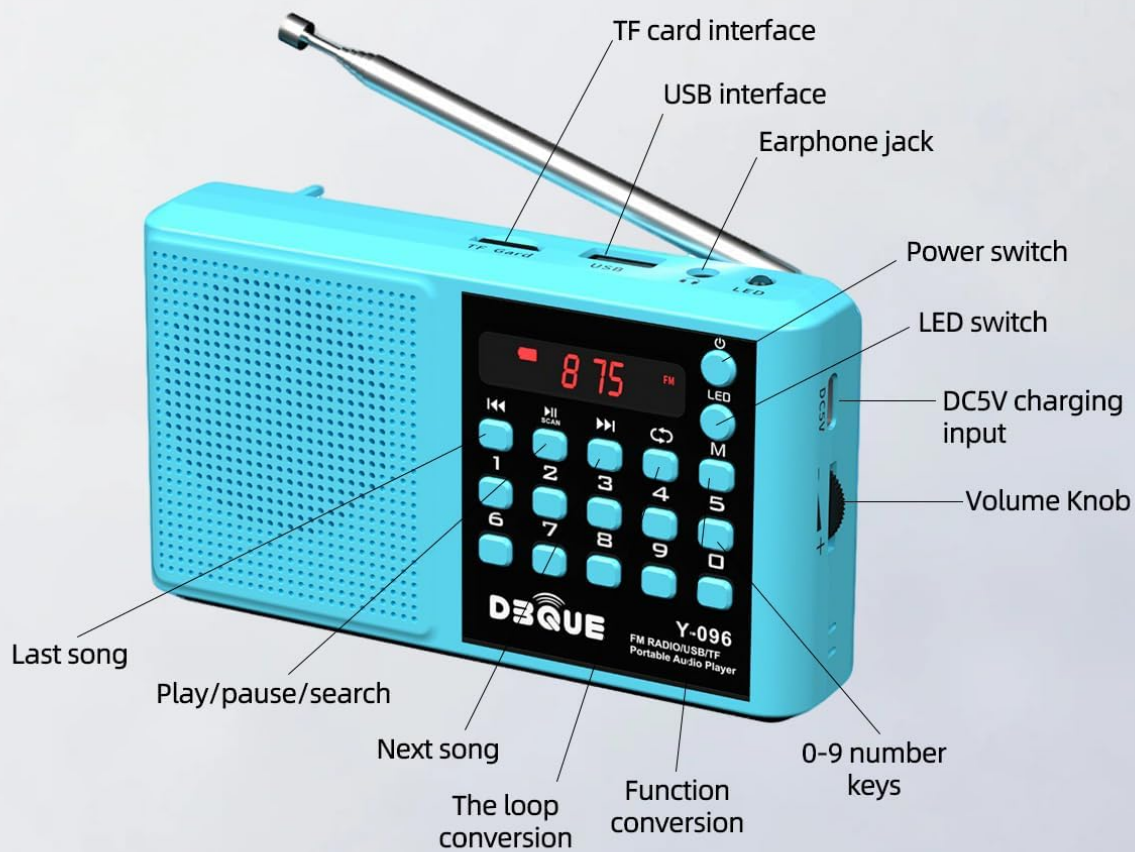
Figure 1: Front Panel and Controls. This image displays the front of the YMDJL Y-096AMBT radio, highlighting its speaker grille, digital display, and control buttons. Key features include the power button, mode button (M), play/pause/scan button, previous/next track buttons, and a numeric keypad (0-9) for direct tuning or track selection. An LED indicator is also visible.
