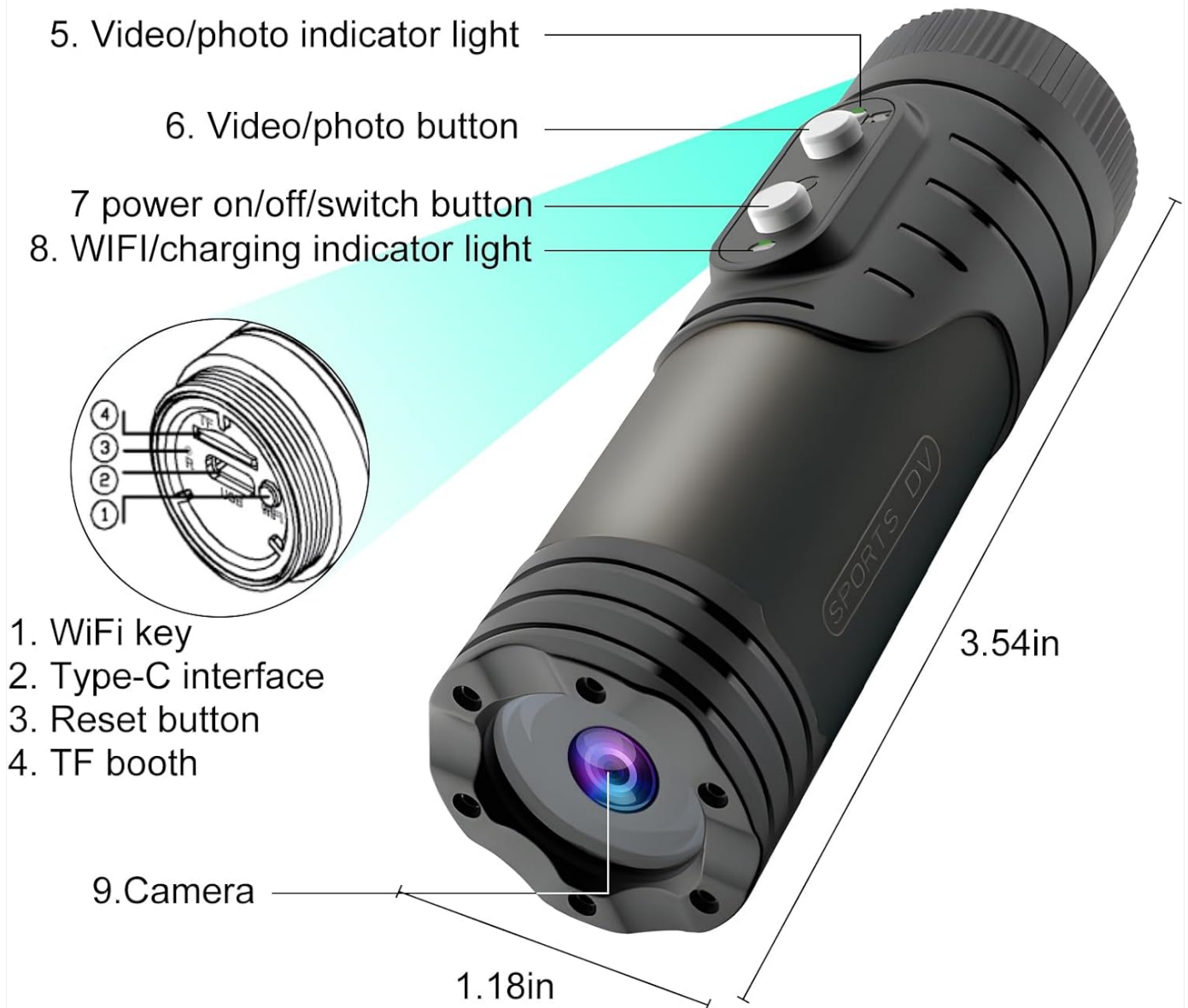
Image 3.1: Detailed diagram of the H81 camera, highlighting its buttons, ports, and indicators.
