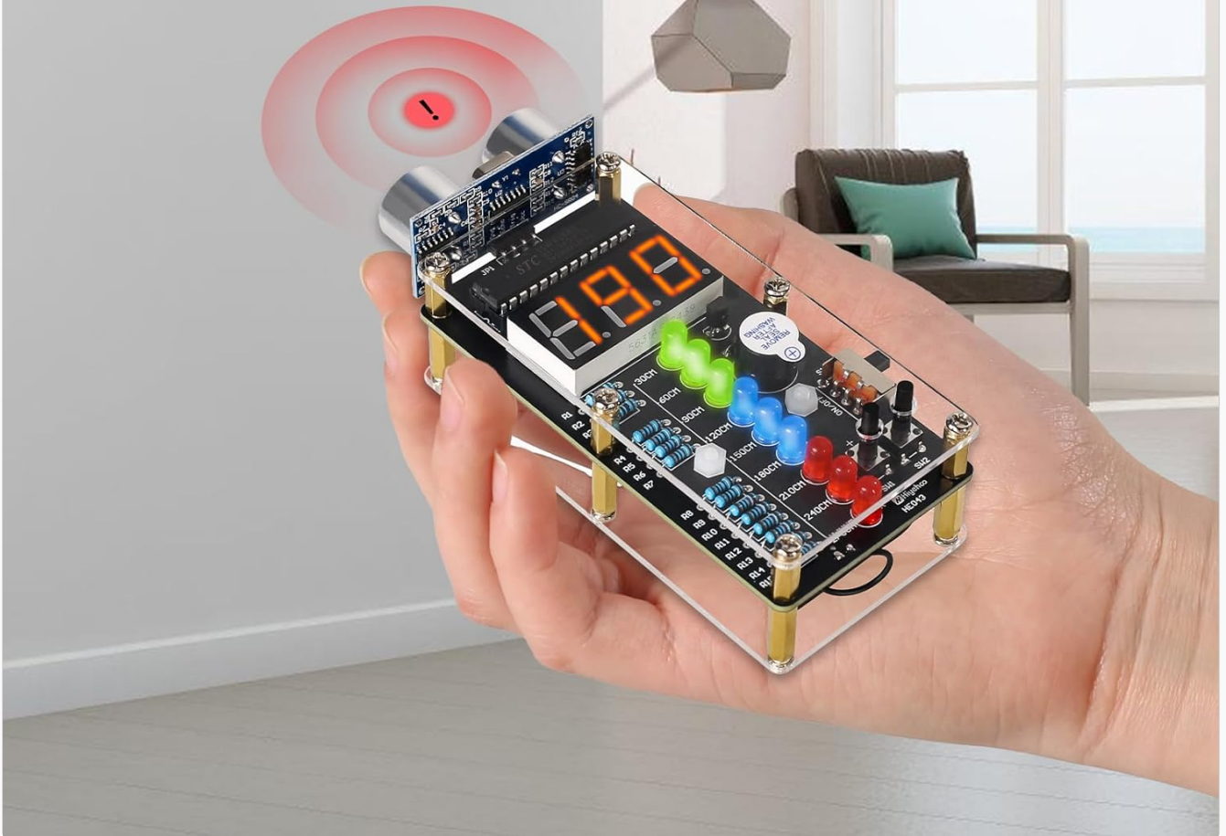
Figure 6.1: Ultrasonic Range Alarm in operation. This image demonstrates how to set the alarm distance using the two buttons, with a visual representation of the alarm being triggered when an object is too close.
