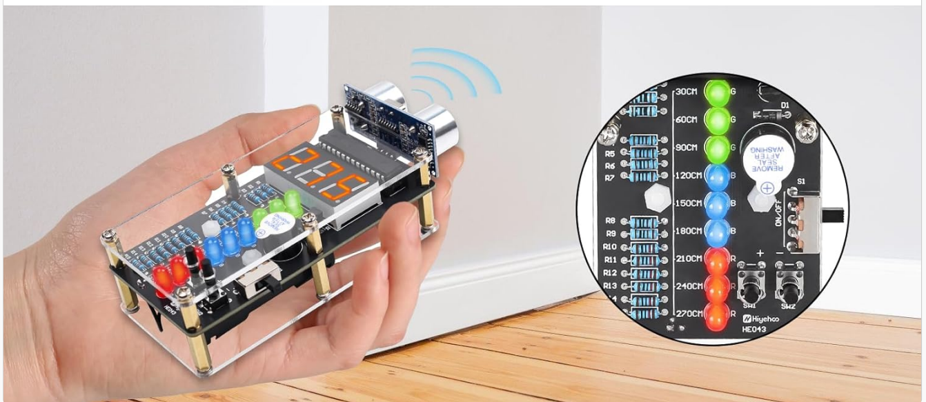
Figure 4.3: Assembled Ultrasonic Distance Measuring Kit. This image shows the completed device held in a hand, highlighting the 3-digit digital tube display and the array of LEDs that light up to provide an intuitive data readout of measured distances.
