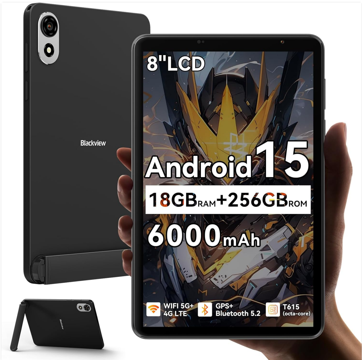
Figure 1.1: Blackview ZENO 1 Tablet highlighting its 8-inch LCD, Android 15, 18GB RAM + 256GB ROM, and 6000mAh battery.
