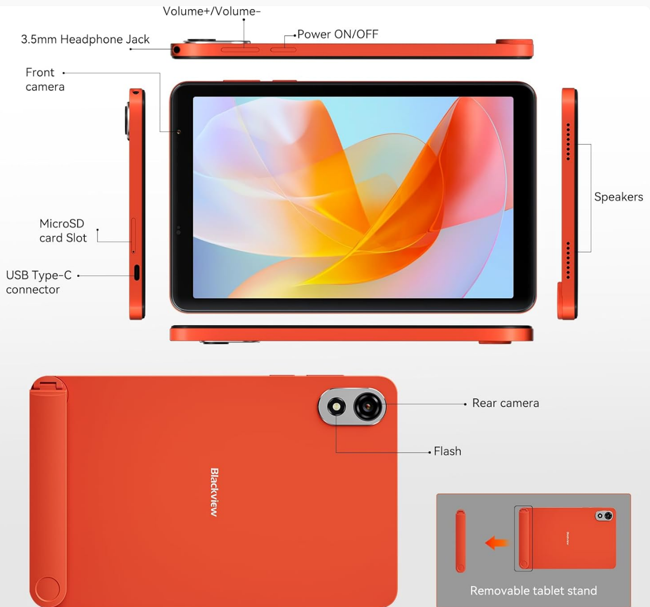
Image: A detailed diagram of the Blackview ZENO 1 tablet, labeling all external components including the headphone jack, volume controls, power button, cameras, microSD slot, USB-C port, speakers, and the removable stand.
