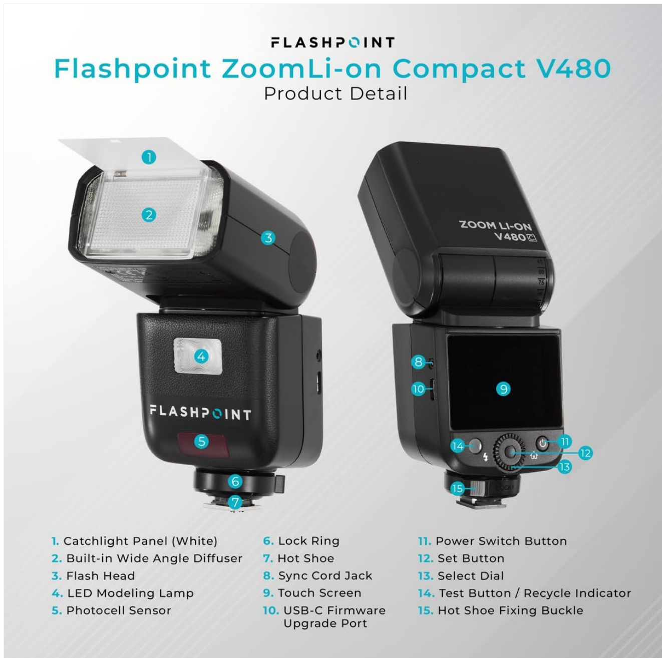
Image 3.1: Front and side view of the Flashpoint V480C with numbered components.
