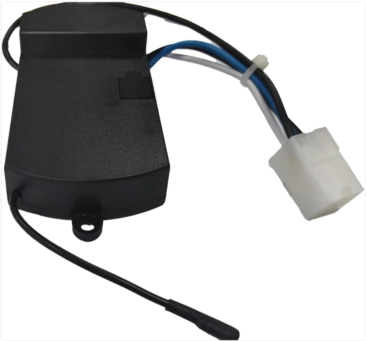
Figure 2: Angled view of the receiver, clearly showing the distinctive square plug connector essential for plug-and-play compatibility with Harbor Breeze Mazon fans.
