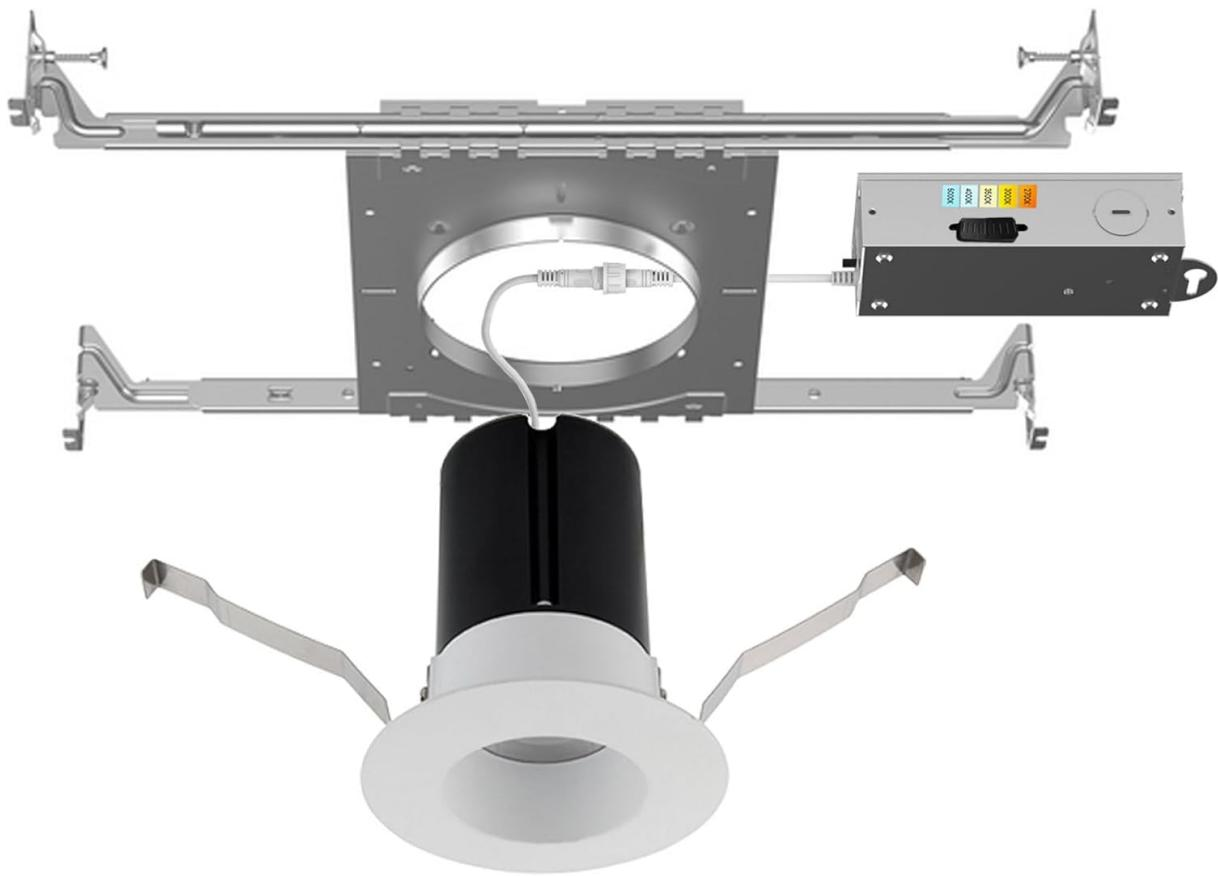
This image illustrates the main components of the WAC Lighting Ion recessed light: the metal frame-in kit, the separate driver box with wiring, and the round LED light engine with retention clips. It shows how the driver box connects to the light engine and how the frame-in kit supports the entire assembly.
