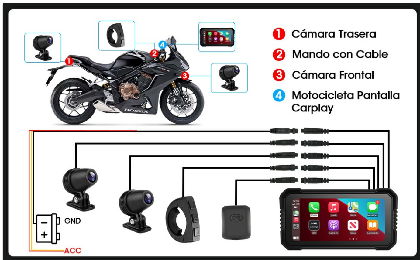
Image: Wiring diagram for connecting the display, cameras, remote, and GPS to the motorcycle's power supply.
