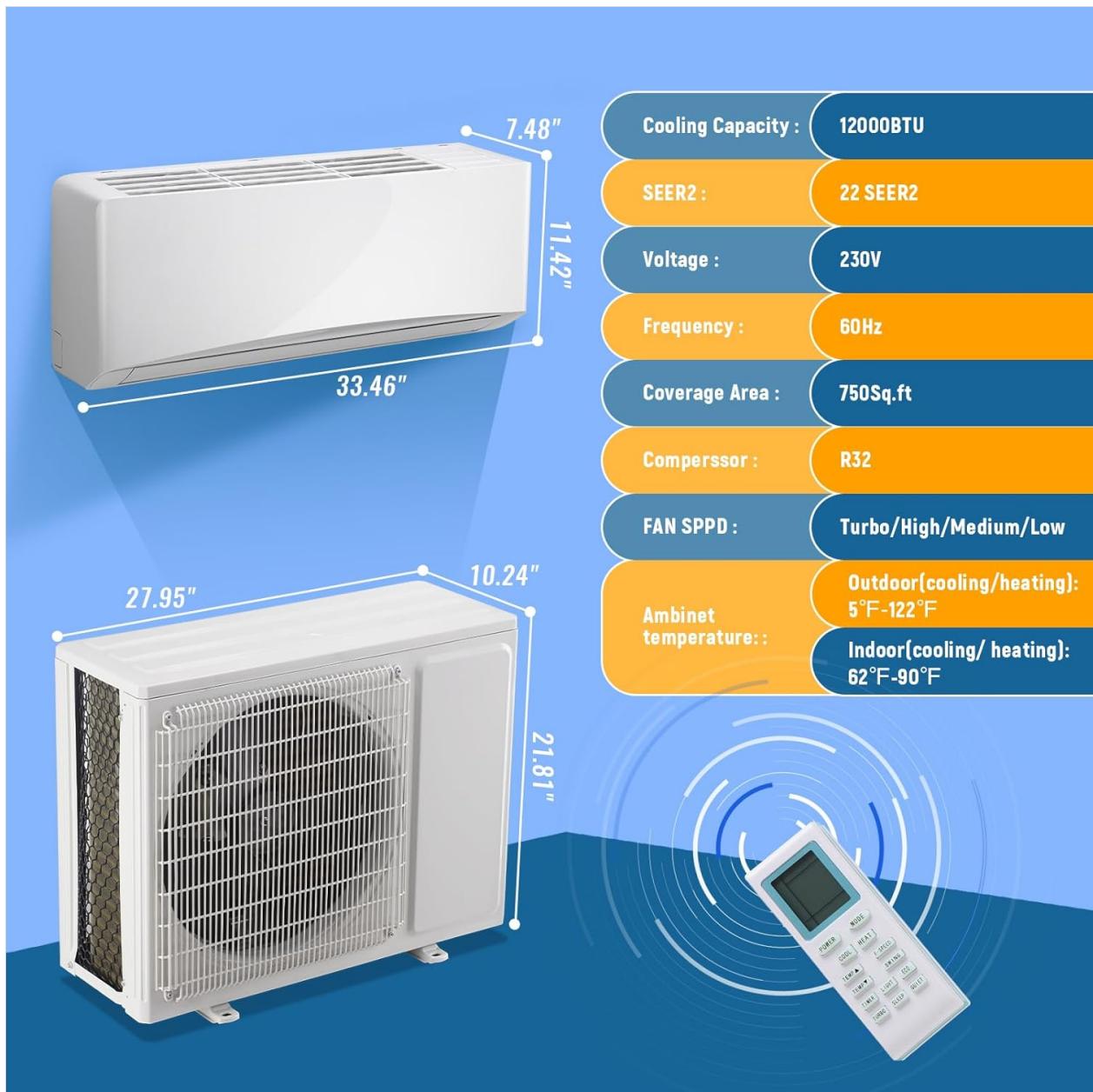
Image Description: This image provides a detailed overview of the product's physical dimensions and technical specifications. It includes measurements for both the indoor and outdoor units, alongside a table listing crucial data such as 12000 BTU cooling capacity, 22 SEER2 rating, 230V voltage, 60Hz frequency, 750 sq. ft. coverage area, R32 refrigerant, various fan speeds, and recommended ambient temperature ranges for operation.
