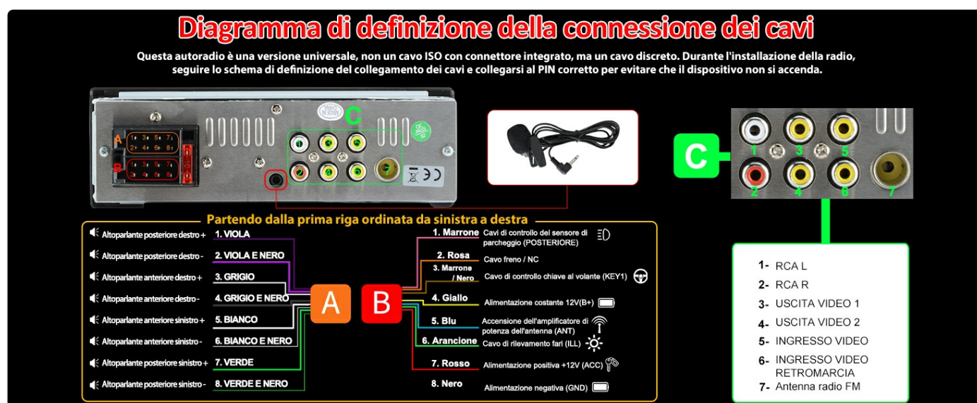
Figure 4.2: Simplified electrical diagram for rear camera and power connections.
