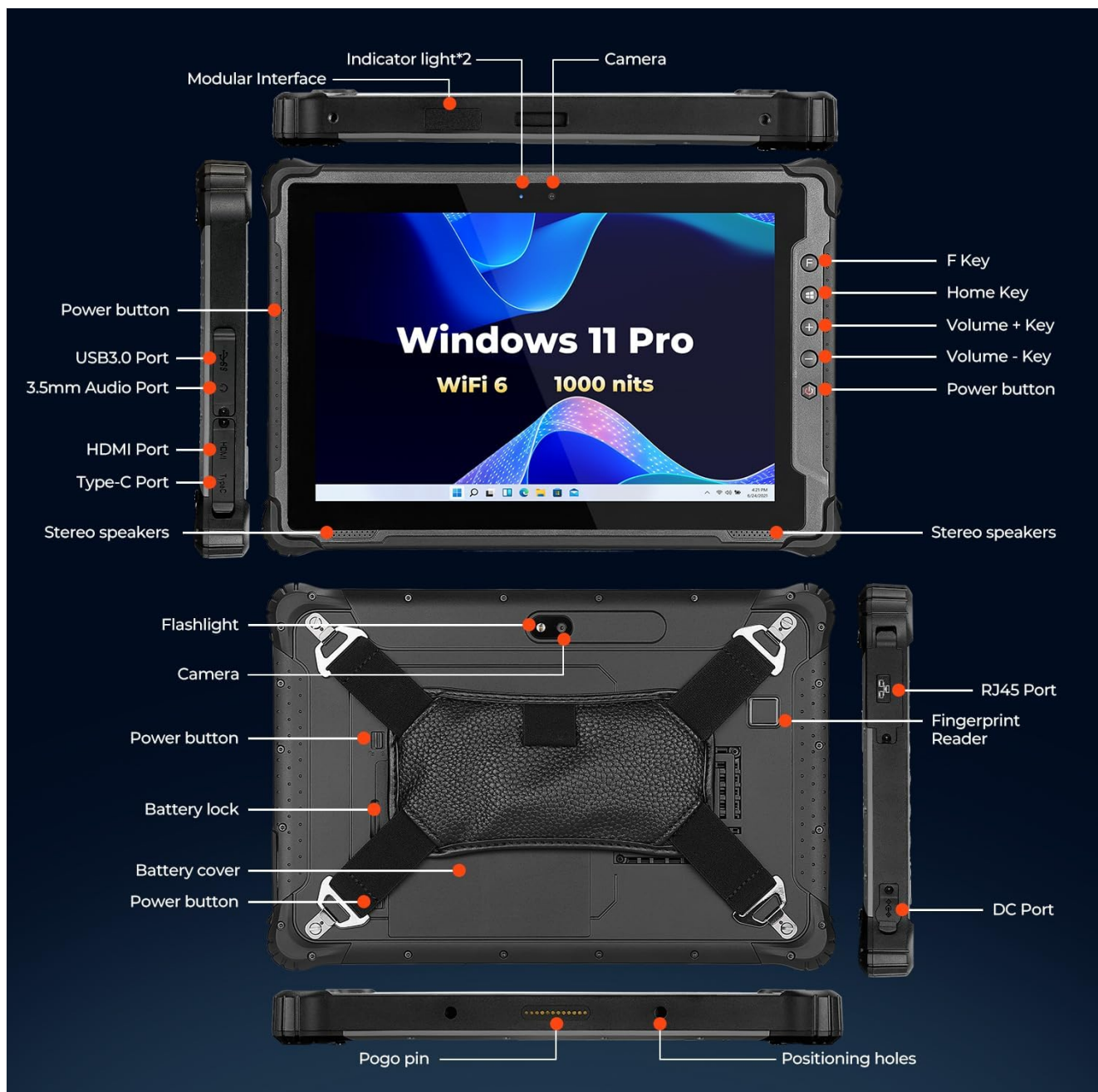
Figure 3.1: Front, back, and side views of the IRT12 tablet with labels for all external components.
