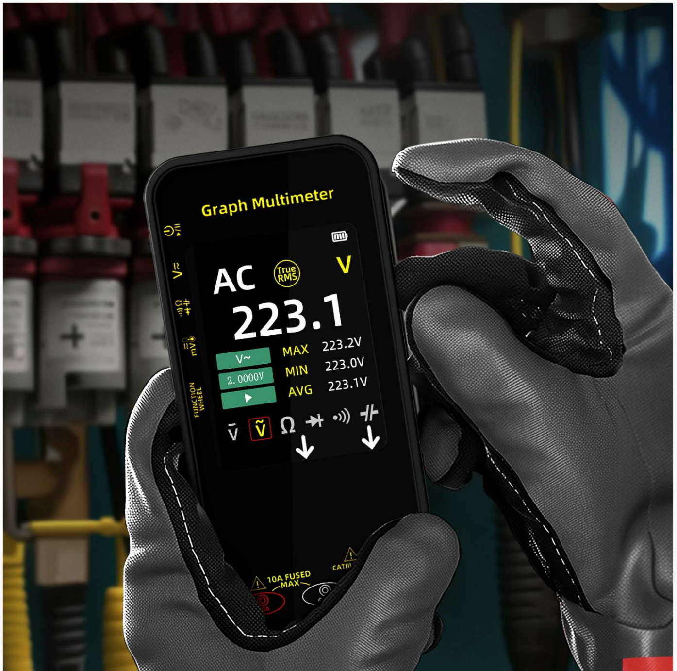
Image 6.1: The multimeter in use, showing an AC voltage measurement on its display.
