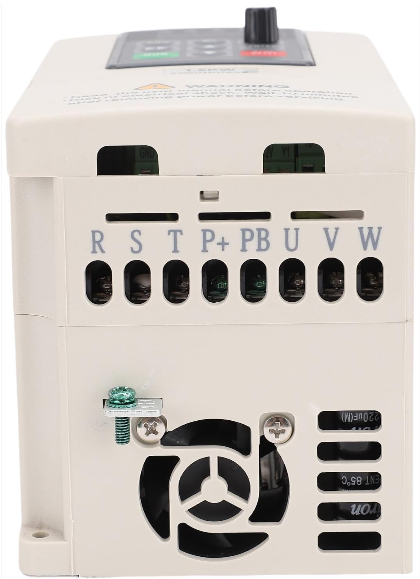
Figure 3.4: Rear view of the inverter, showing the main power input (R, S, T) and motor output (U, V, W) terminals, along with grounding point.
