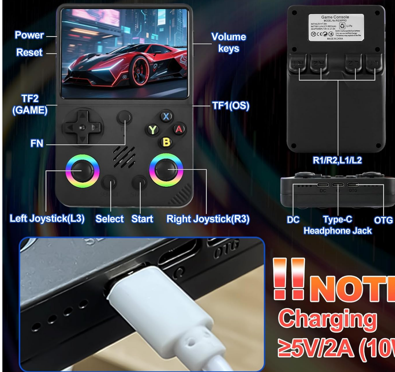
Image 4.1: Front, back, and top views of the RG36PRO, labeling key components such as Power/Reset, Volume keys, TF1(OS) and TF2(GAME) card slots, FN button, Left/Right Joysticks (L3/R3), Select/Start buttons, DC port, Type-C Headphone Jack, and OTG port.
