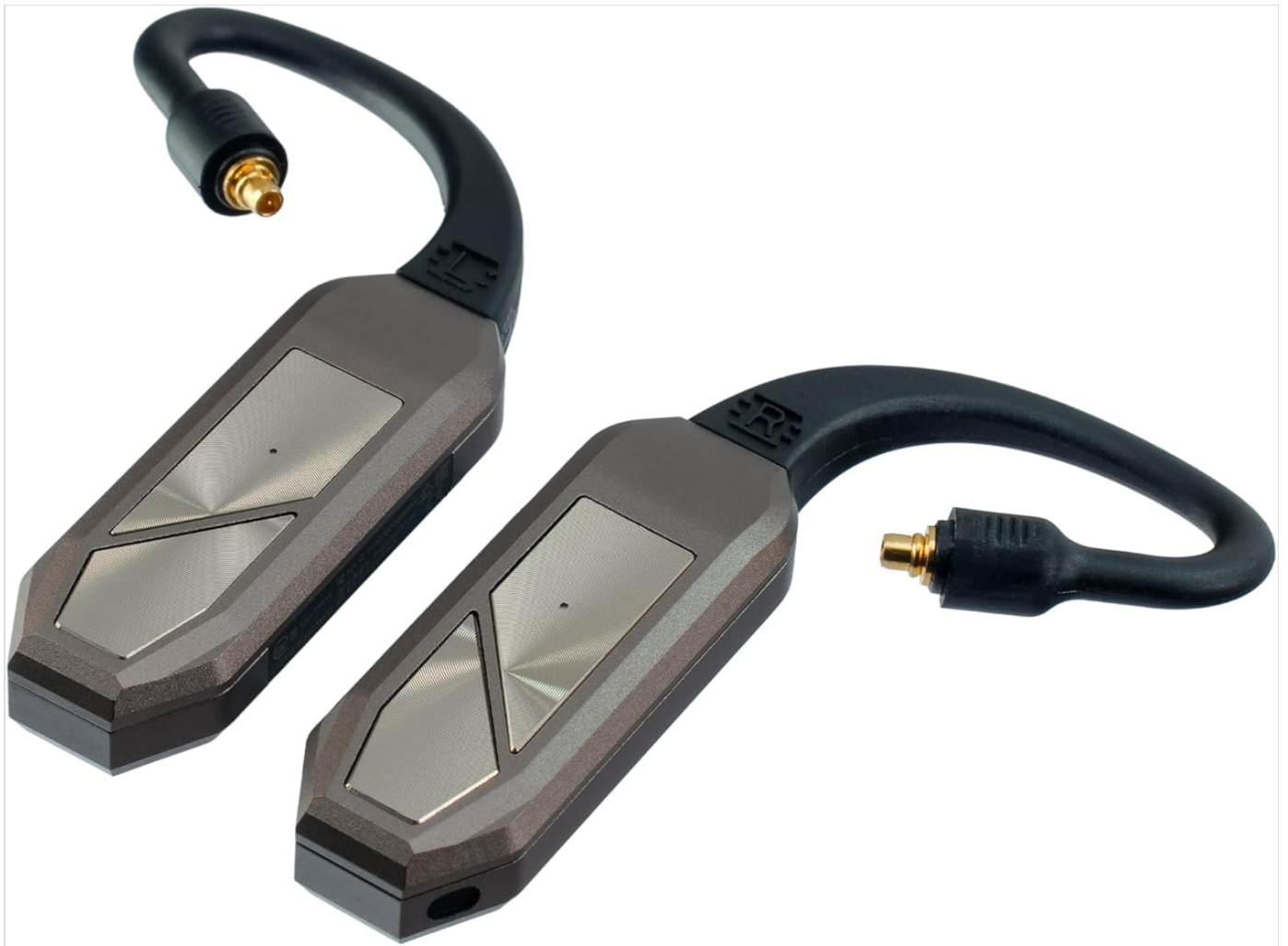
Image: A GO Pod Max unit with its ear loop detached, demonstrating the interchangeable connection system.
