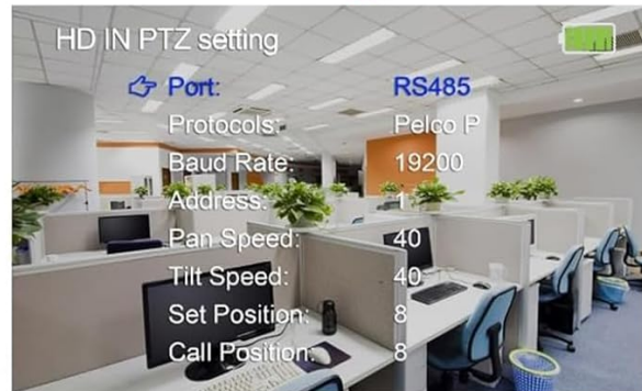
Figure 7: Auto HD function recognizing camera type and displaying PTZ settings.
