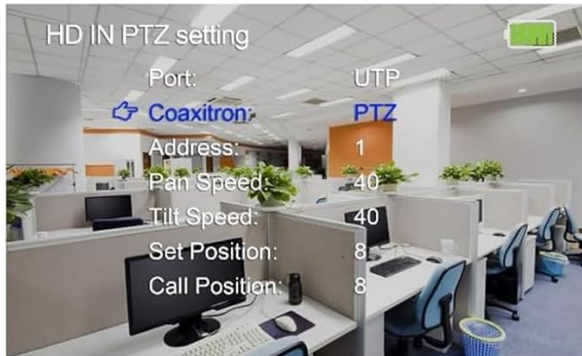
Figure 7: Auto HD function recognizing camera type and displaying PTZ settings.
