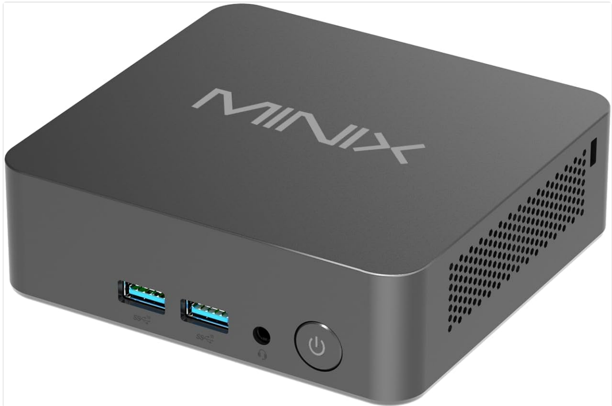
Image: Front view of the MINIX NUC150 Mini PC, showing two USB 3.0 ports, an audio jack, and the power button.
