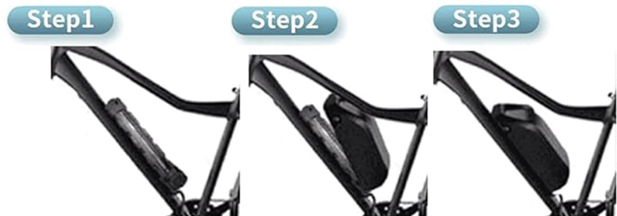
Figure 4: Step-by-step installation guide for the battery. This diagram illustrates how to attach the battery mount and then slide the battery onto it.
